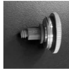
NG Position: Plastic Ring is next to the cap
