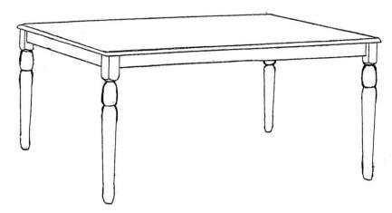
ATTACH THE TABLE LEGS (B) TO THE CORNER BLOCK WITH HEX SCREW (C) SPRING WASHER (F) AND FLAT WASHER (D). TIGHTEN THE HEX SCREW (C) BY USING THE HEX WRENCH (E).
