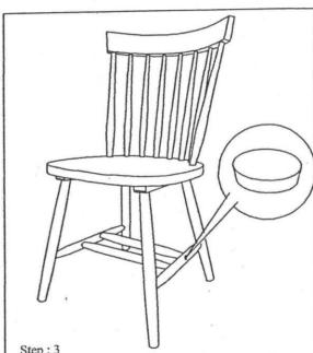
Please tighten all the JCBC Bolt & Screw then insert the Wood Button (F) to the bottom stretcher for cover the hole.
