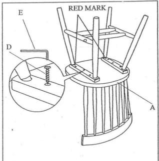
Position the frame assembly into the bottom of chair seat. Align and tighten bolt chair seat and frame using the JCBC Screw (D) with Allen Key (E).
