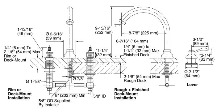
\*Dimension allows 1/4" (6 mm) handle adjustment during handle trim installation.
