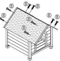
Place the Ridge Cap onto the Shingle Roof Panels and secure using 4 - 1" screws (C). Attach 3 star shaped bolts (D) on the
