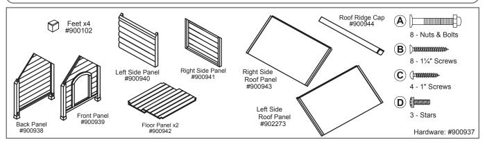
Step 1 Connect the Front Panel and the Back Panel to the Left Side Panel and right Side Panel using the 8 - 2%" Nuts and Bolts (A).
