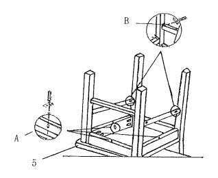
There are no pre-drilled holes to attach the seat
