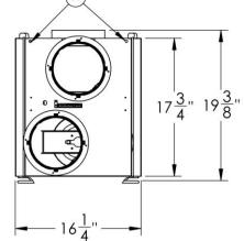
Unit is reversible, 2 doors are removable if required for access to core and routine maintenance
