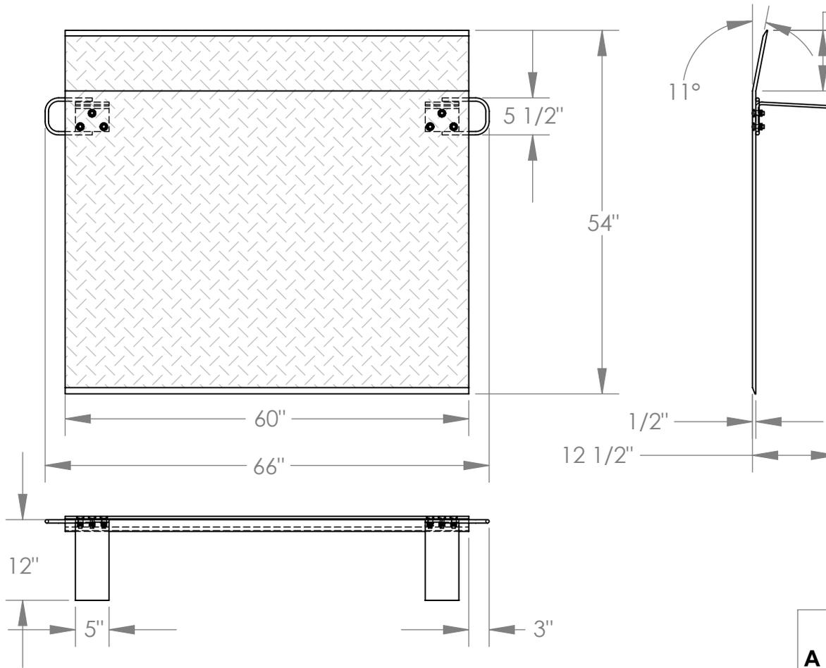
NOTE: BEND OR CROWN IS 11° AND LOCATED 9" FROM EDGE OF DOCKPLATE
