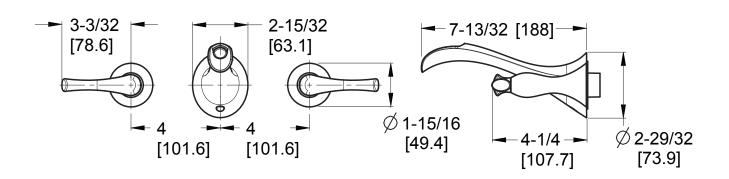
Ø1 Min to Ø1-1/2 Max. Deck Hole Openings
