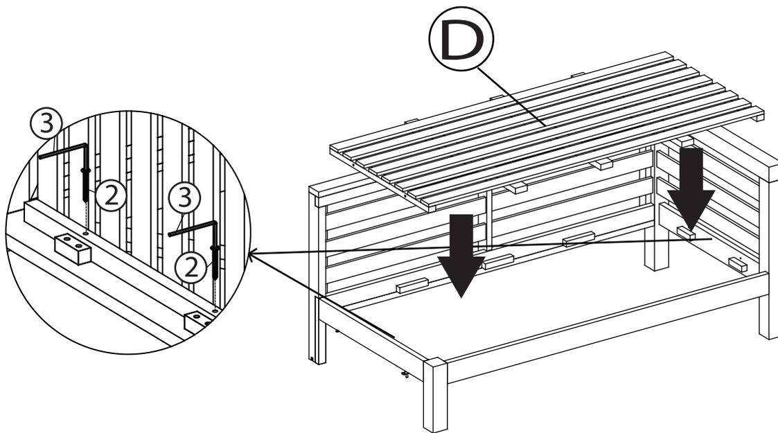
Attach the Seat Panel (D) into the Right Chair as shown in picture above.
