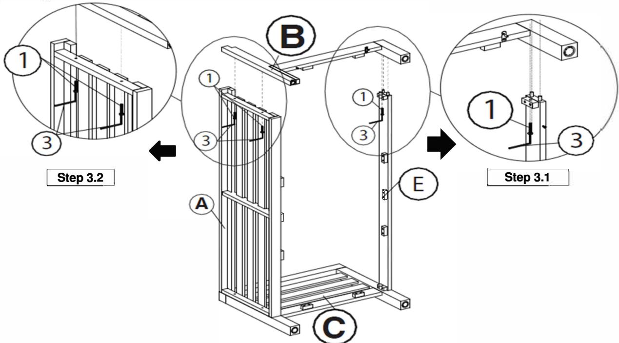
Place Left Arm Panel (B) onto the assembled frame from Step 2
