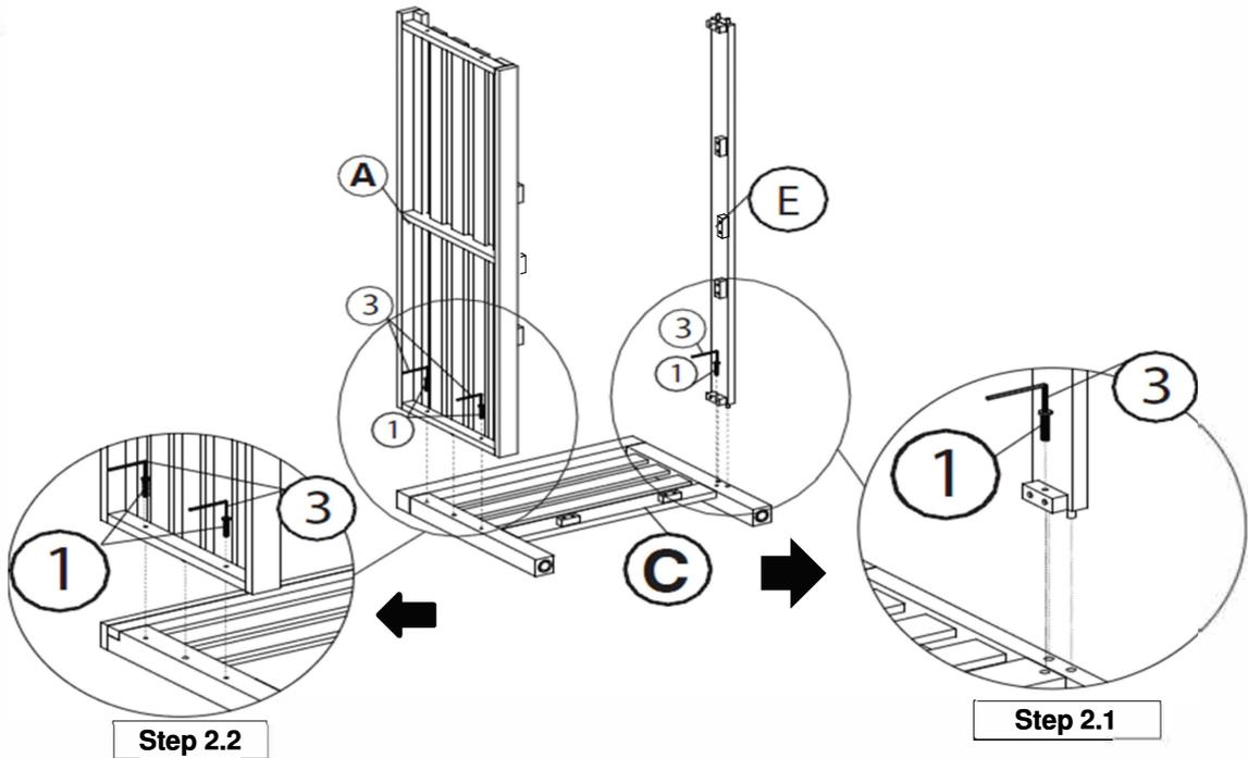
Place the Right Arm Panel (C) with inside face skywards onto a clean, soft surface to avoid any scratches or damages to the product.
