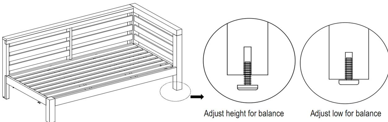
Adjust Pre-installed Levellers
