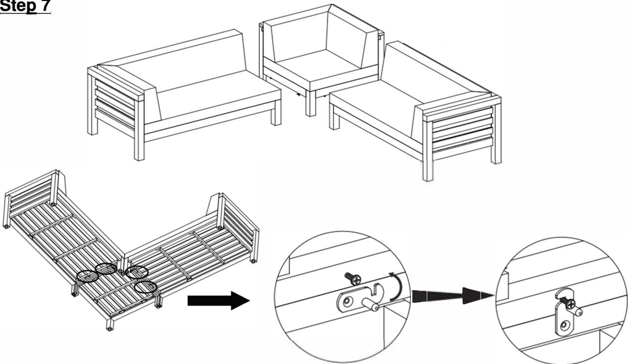
Note: This is optional step in case we want to connect all chairs in a set together and should be done before placing cushion
