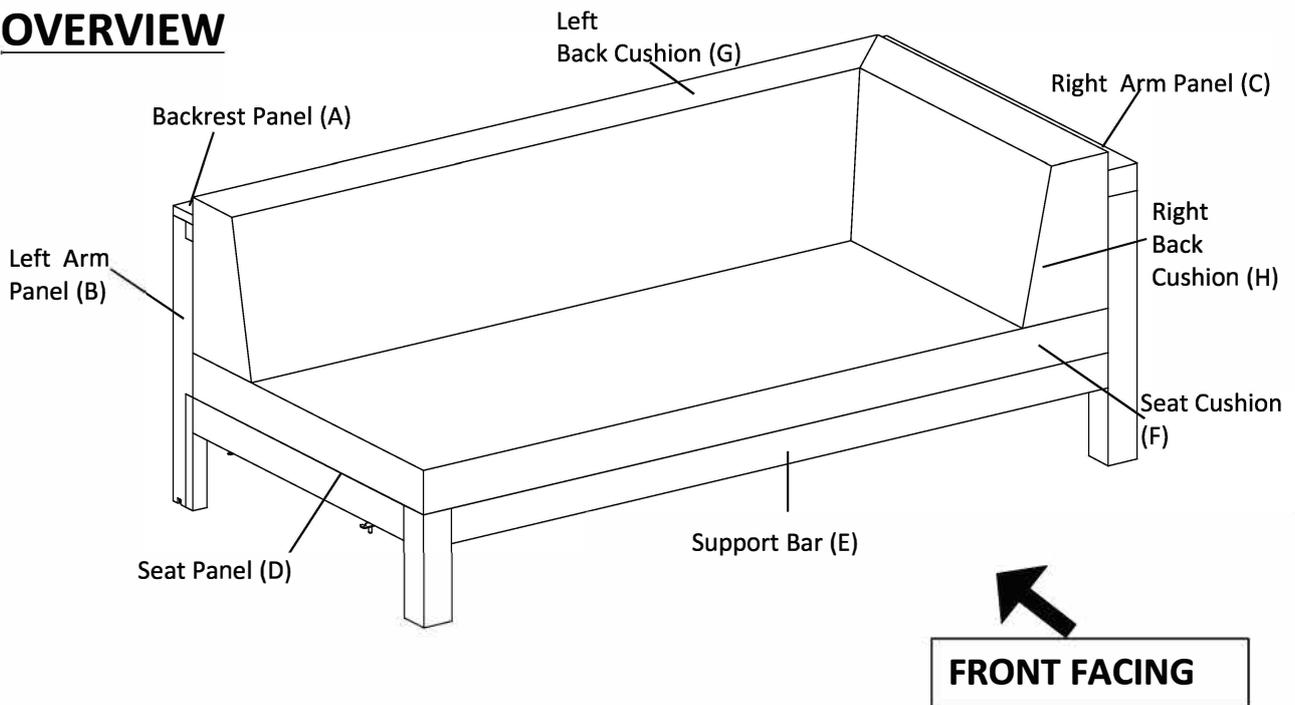
This Right Chair has multiple parts and may require up to 30 minutes to assemble. To give you an overview of the Right Chair parts, the above picture is to help you put the various parts into perspective. Please read through the instructions herebelow to familiarise the parts and steps before assembly.
