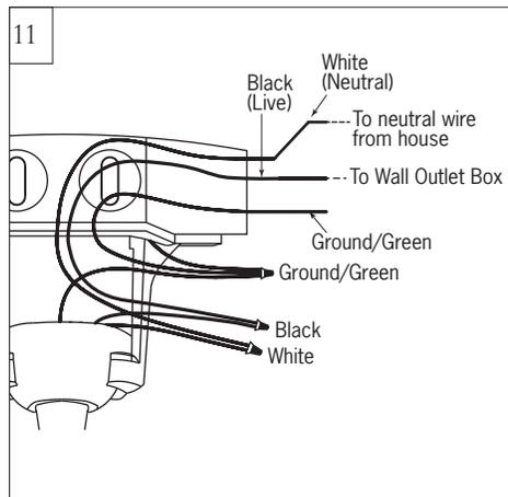
**Refer to page 6 for wiring, installation and operation of Wall controller. Do not operate the fan or light until it is installed completely**
