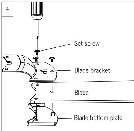
Install a blade bracket onto blade with a blade bottom plate using set screws provided. Repeat this process for remaining blades.
