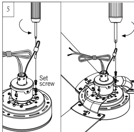
Put motor assembly on a suitable area of paper pulp. Remove the blade set screws from motor. Install the blade assembly to motor using the set screws. Tighten screws securely. Repeat this process for remaining blade assemblies.
