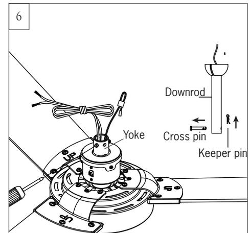
Partially loosen downrod set screws from yoke at top of motor assembly. Remove preassembled cross pin and keeper pin from downrod. Keep parts.
