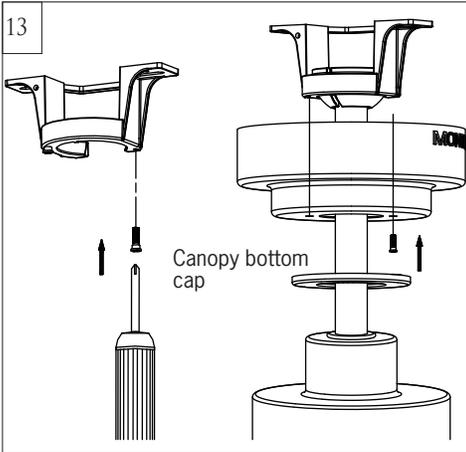
Partially loosen one and remove one preassembled screw from mounting bracket. Save screw.
