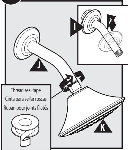
Slide Shower Arm Flange (I) onto Shower Arm (J). Wrap Shower Arm (J) with thread seal tape. Thread Shower Head (K) onto Shower Arm.
