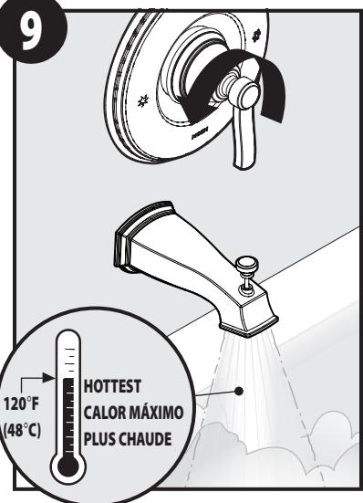
Turn handle on to test hot water temperature. Turn off handle if desired water temperature has been met. Hot water temperature should not exceed 120°F.
