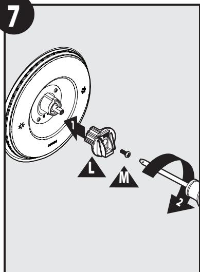
Install Handle Adapter (L) onto cartridge stem with Handle Adapter Screw (M).
