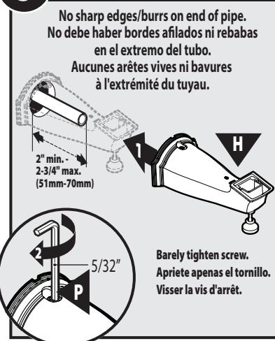
1. Install Tub Spout (H) upside down onto pipe.
