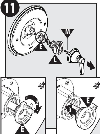
Remove the Handle (M) and vHandle Adapter (K). Note the position on the stop. Position the Adjustable Temperature Limit Stop (D) so the Handle stops at the position. This prevents the Lever from being turned into an unsafe temperature.
