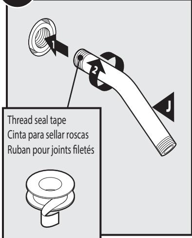
Wrap thread seal tape around Shower Arm (J) threads. Screw Shower Arm into connection in wall.
