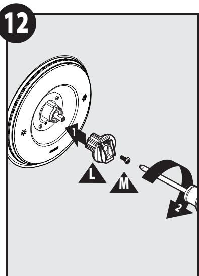
After setting the adjustable temperature limit stop to the desired position, reattach the Handle Adapter (L), Adapter Screw (M), and Handle (N). Make sure ridges on back of (L) are to the left of the tab on (E).
