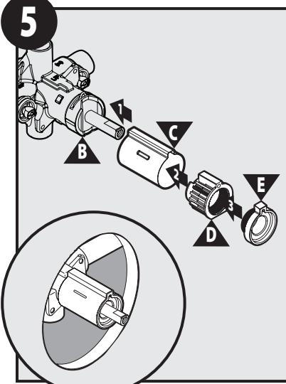
1. Slide Stop Tube (C) onto valve (B).
