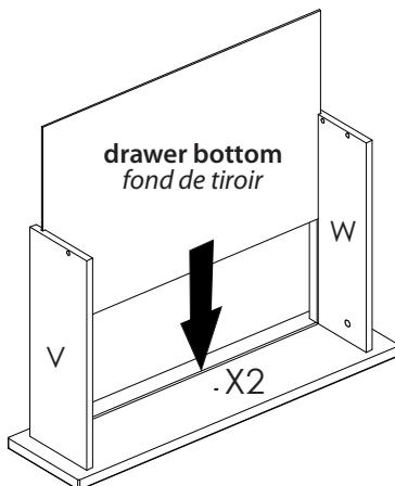
Drawer bottom must enter into the groove located on panel X2
