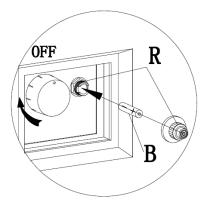
Remove the Electronic Ignitor Cap (15) on the electronic Ignitor (15) by unscrewing and slide the Battery (B) into the battery slot (15).
