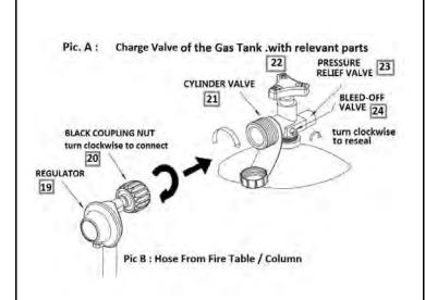
Step 1 : Plug the Black Coupling Nut on the Regulator to the Cylinder Valve.
