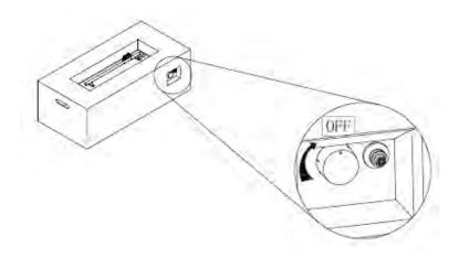
1. Check that the Control Knob (14) for the gas supply system is turned to the "OFF" position before starting any assembly.
