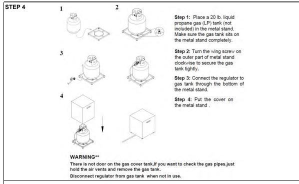
4. Place the 20lbs Propane Gas Tank (not included) into the Tank cover (08). Make sure the Propane Gas Tank is placed completely into the Tank cover (08).
