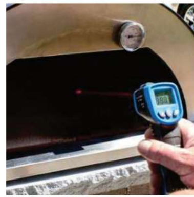
Once the Cooking Stone reaches 644°F or higher, you are ready to start cooking entrees, desserts, and pizzas. (Do not overheat the oven.)
