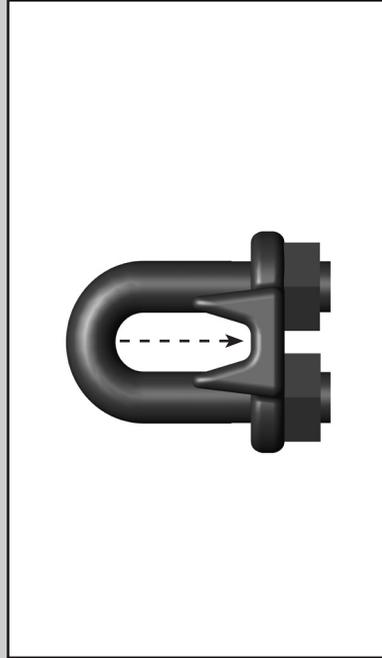
Loosen the two nuts on the wire clamp and slide the clamp open. Thread the end of the cable up through the wire clamp.
