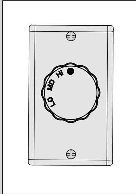
Reattach the knob onto the wall control and turn it to the left for the OFF position.
