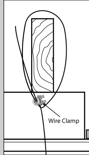
Wrap the braided cable around the support brace once, creating a complete circle. Thread the end of the cable through the bottom of the clamp again so the excess cable hangs out the top. Be sure to remove any slack from the cable.
