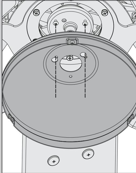
Wrap the keyhole slots in the upper switch housing around the screws and twist counterclockwise.
