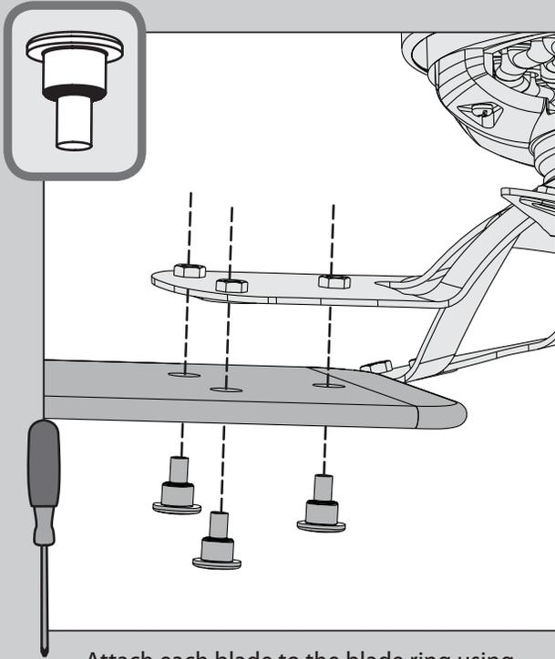
⊗ Attach each blade to the blade ring using three blade assembly screws, found in the ▲ hardware bag.
