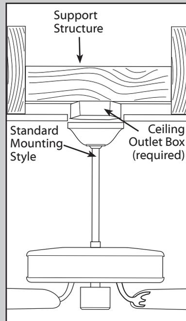
Use **Standard Mounting** to hang the fan from a flat ceiling.
