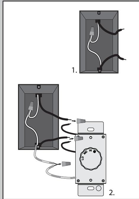
Using the wire connectors, connect each black wire from the wall control to a black wire from the switch box. Connect the green with yellow stripe wire to the grounding wire from the switch box.
