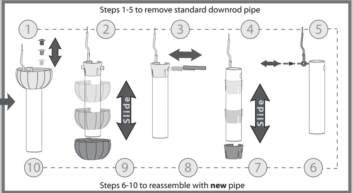
**Tip:** If you have difficulty feeding the wires through the downrod, try taping the wires to a thin dowel rod, then drop the dowel rod and wires through the downrod. Be sure to remove all tape once the wires are fed through to the other side.
