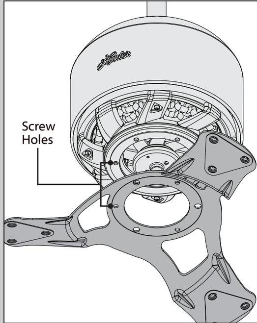
Lift a blade ring to the motor assembly and align the screw holes.
