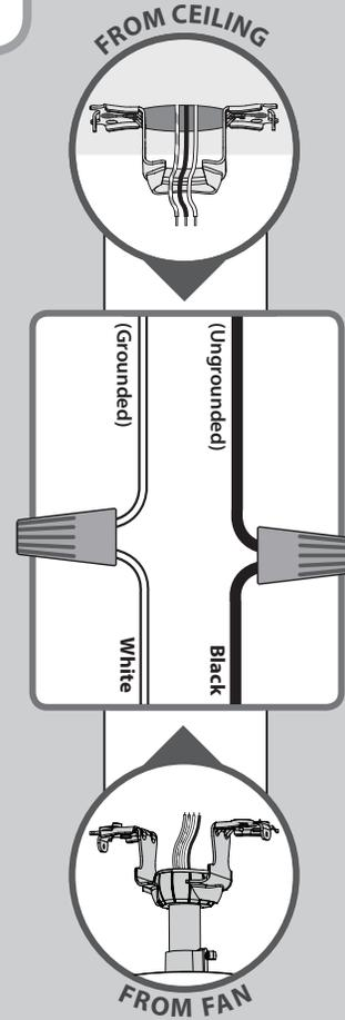
Using the orange wire connectors from the ★ hardware bag, connect the black wire (ungrounded) from the ceiling to the black wire from the fan. Connect the white wire (grounded) from the ceiling to the white wire from the fan.
