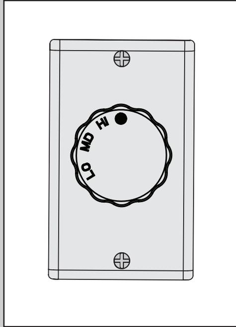
The knob on the wall control unit controls power to the fan. The fan has four speed settings in sequence: high, medium, low and off.
