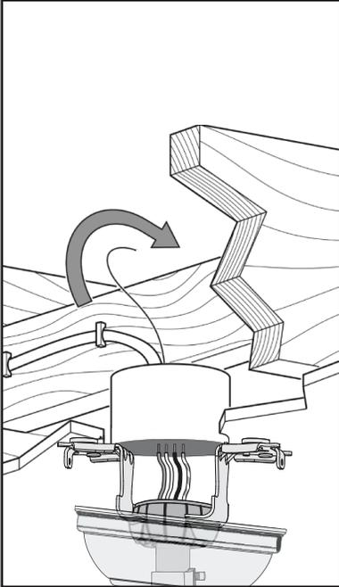
Insert the end of the braided cable through the ceiling bracket and one of the holes in the outlet box into the ceiling. Access the support brace in the ceiling. You may not be able to do this from below the ceiling depending on your installation site.
