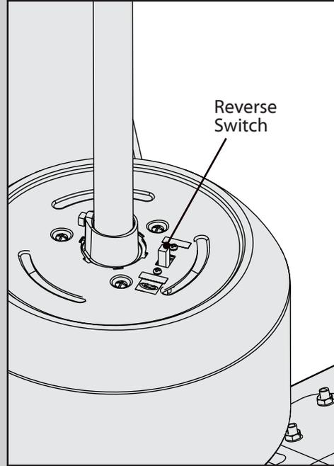
To change the direction of air flow, move the reverse switch to the opposite position.
