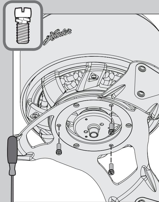
Install three blade assembly screws, found in the ☒ hardware bag.
