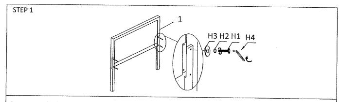
**Step 1:** Attached Headboard post (L/R) to the headboard using flat washer (H3), Lock washer (H2) and Allen bolt (H1).
