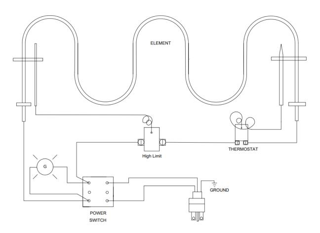
WIRING DIAGRAM - MANUAL RESET
