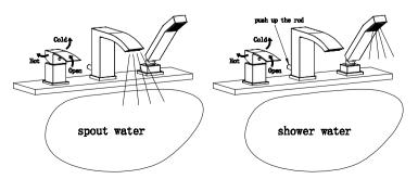
(6) After the installation, you must test the faucet, check the spout and the shower is work correct!
