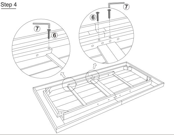
Loosely affix by using the Screws  $(\widehat{\mathbb{G}})$  and Allen Key  $(\widehat{\mathcal{T}})$  as shown in the picture. Repeat the same process with the other Support Bar (C). **Only loosely tighten the Screws.**
