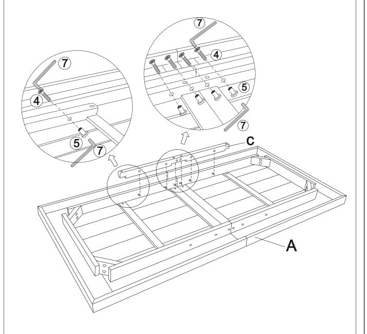
Place Support Bar (C) to the housings of Table Top (A), secure by using the Short Bolts (4) with Sleeve Nuts (⑤), as shown in the picture.
