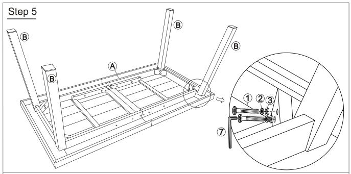
Affix loosely the Legs (B) into the mounting position at the corners of the Table Top (A), using the Long Bolts (1) with Spring Washers (2), Flat Washers (3), as shown in the picture. Repeat the same process with the other Legs (B).
