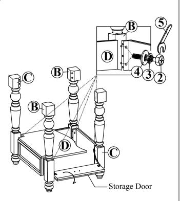
Step 1: Open the storage door of the Table Storage (D). Attach the LSF Front Leg (or RSF Back Leg) (B) and the RSF Front Leg(or LSF Back Leg) (C) to the Table Storage (D) by inserting Short Bolt (2), Lock Washer (3), Flat Washer (4), tighten with Wrench (5). Do not fully tighten.
