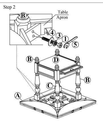
Step 2: Place the Table Top (A) upside down on a piece of cloth or carpet to prevent finish from scratching.
