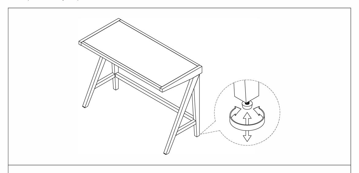
STEP 5 ADJUST THE ADJUSTER BOLT THAT HAS ALREADY ASSEMBLED TO THE LEGS TO STABILIZE YOUR UNIT
