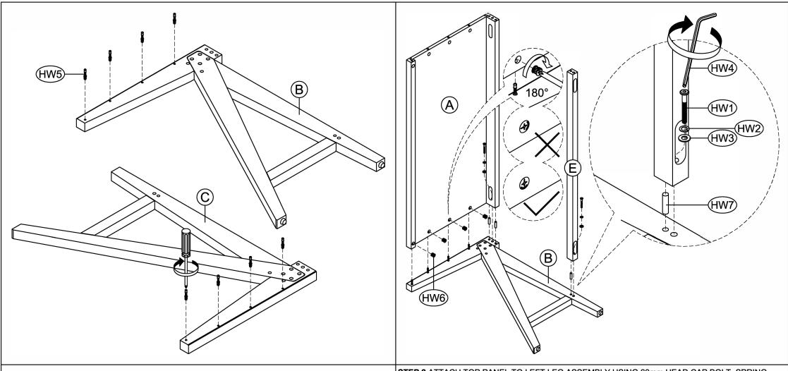
**STEP 1** INSERT CAMBOLTS INTO PRE-DRILLED HOLES IN LEFT AND RIGHT LEG ASSEMBLIES, THEN TIGHTEN. SCREW-IN CAMBOLTS MUST BE SCREWED DOWN FLUSH.
