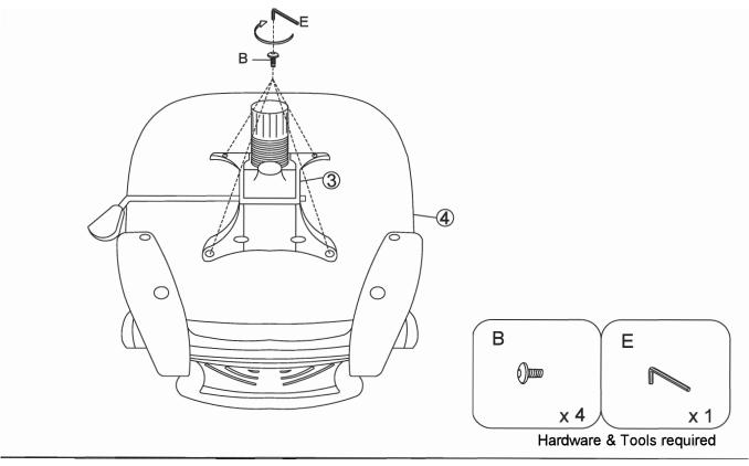
STEP 6: Insert assembled top unit from Step 7 onto the Cylinder Column (Part 2) as shown.
