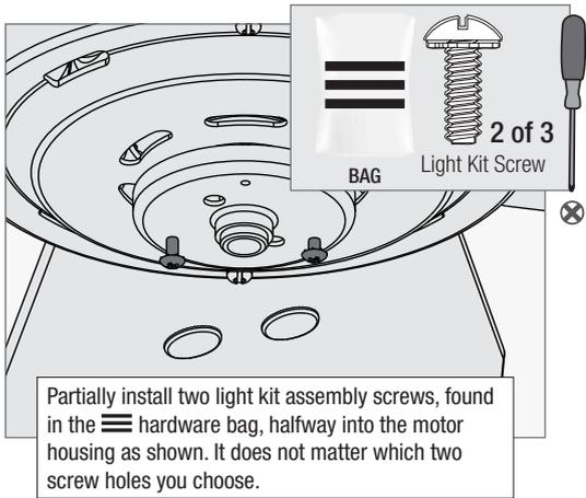
Partially install two light kit assembly screws, found in the
