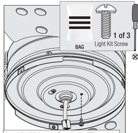
Insert the third screw, found in the
