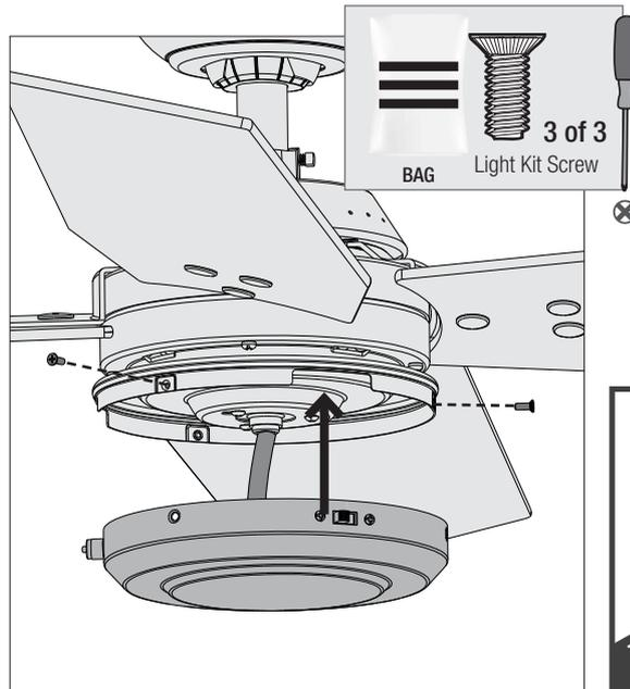
Lift the lower switch housing until its screw holes are aligned with the screw holes in the upper switch housing. Install the three switch housing screws, found in the
