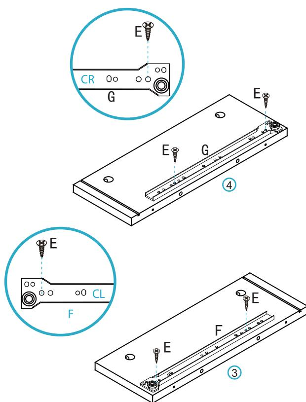
**EN** Please find the exact hole for installation, otherwise it will be misaligned. The screws on the drawer slide must be leveled, otherwise it will affect the smoothness of the drawer.
