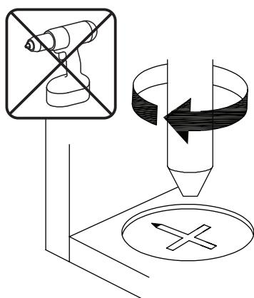
**EN**\_Turn cam lock clockwise to tighten.
