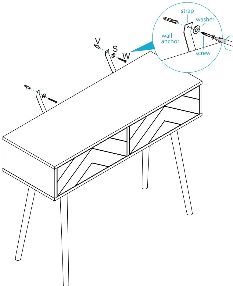
**EN** If it is a solid wall, please use expansion and self-tapping screws, if it is a wooden wall, only use self-tapping screws, please do not overtighten the screws
