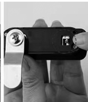
5. Reset the lever to the initial position
