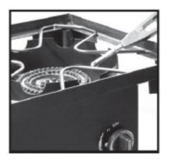
**STEP 3: •** Light burner; rotate knob(s) from HIGH to LOW. You should see a smaller flame in LOW position than seen on HIGH. Always check flame prior to each use. The air damper mounted on the back of your burner helps to control the amount of primary air that mixes with the LP gas. A blue flame with little or no yellow flame provides the best heat. Adjust the air damper by turning it clockwise or counterclockwise until the desired flame is achieved.
