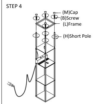
Place frame (L) onto the short poles (H) and tighten with screws (B). Then put the caps (M) onto frame (L) over the screws (B).
