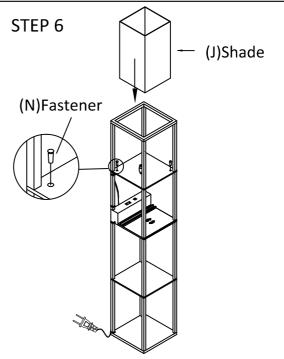
Place shade (J) onto USB board (G) and secure with fasteners (N).
