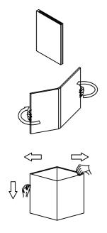
Press by hand along folded edge of shade (J) to expand the shade (J) into its full size.
