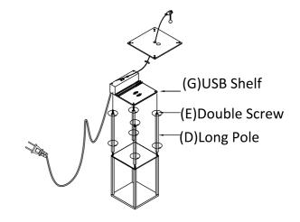
Screw poles (D) clockwise into shelf (F). Then screw the four poles (D) and USB shelf (G) together with the double screws (E) until tight.
