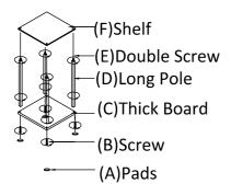
Begin assembly with the base of the lamp. Screw poles (D) clockwise into thick board (C) with screws (B) until tight and cover them with pads (A). Then screw four long poles (D) and shelf (F) together with double screws (E) until tight.
