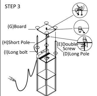
Screw poles (D) and USB shelf (G) together until tight and then insert double screws (E) into poles (D) and screw tight. Set the socket on USB board (G) and drop the pull chain directly through the hole and screw the socket until tight. Then place USB board (G) onto the poles (D).
