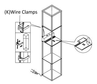
Insert the wire into wire clamps (K) and then attach the clamps (K) to the poles, using one clamp per level.
