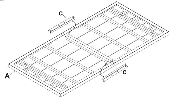
Place Support Bar (C) underside of long apron of Table Top (A) as show in picture above.
