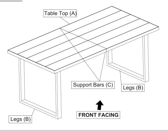
This Table has multiple parts and may require up to some 30 minutes to assemble. To give you an overview of the table, the above picture is to help you put the various parts into perspective. Please read through the instructions here below to familiarise the parts and steps before assembly.
