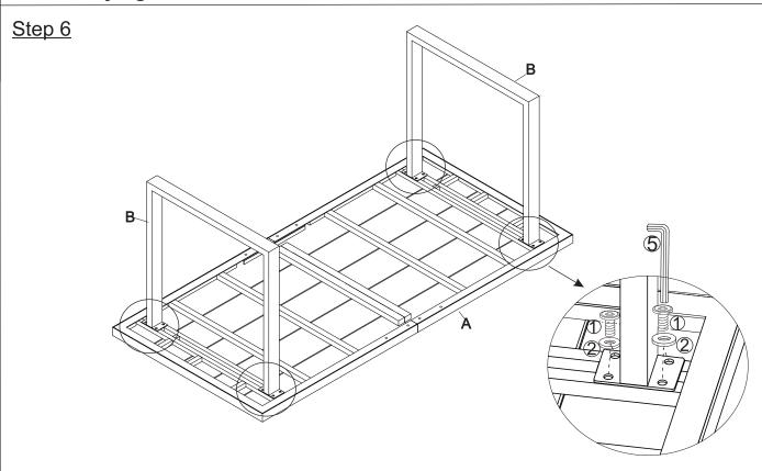
Attach the Legs Frame (B) to the Table Top (A) using the Bolts (1) with Washers (2) and Allen Key (5) as shown in the picture.
