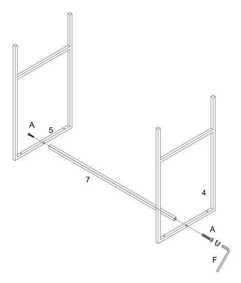
Using bolt (A) secure parts (4,5) into part (7) with hex key (F) as per diagram.
