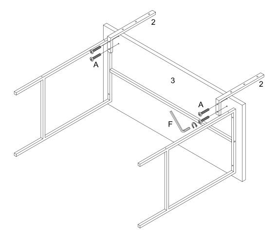
Using bolt (A) secure part (2) into part (3) with hex key (F) as per diagram.
