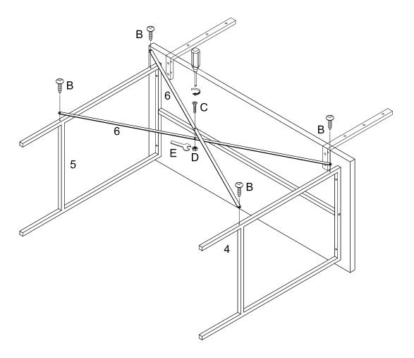
Using screw (B) secure part (6) into parts (4,5) with Philips head screwdriver, then using bolt (C) secure part (6) into nut (D) with hex key (E) and Philips head screwdriver as per diagram.
