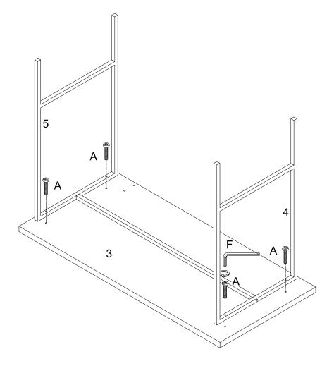
Using bolt (A) secure parts (4,5) into part (3) with hex key (F) as per diagram.
