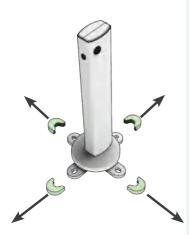
Note: Remove four black plastic sleeves before installing the base tube.
