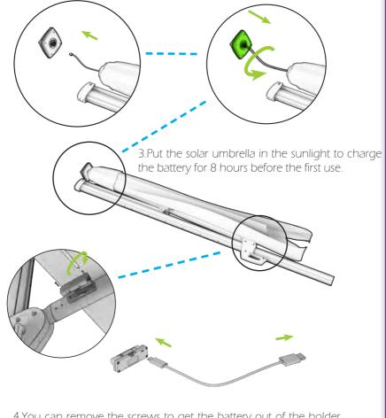
4. You can remove the screws to get the battery out of the holder, then charge it with USB wire.
