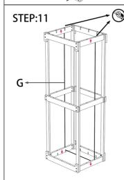
Finally, pass five ropes through the holes and tie them to complete the installation. After installation, all the labels are on the outside of the product, and then you can remove the stickers.
