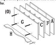
Insert 10 cam locks (L) into predrilled holes on the sides of assembly that line up with cam screws in side panels (I/J). Attach side panels (I/J) to assembly. Turn cam locks (L) in assembly to lock assembly together.
