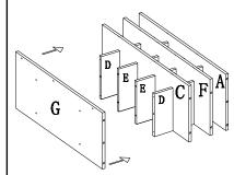
Screw bottom panel (G) into place using long screws (O). Insert 2 cam locks (L) into predrilled holes in moulding (H). Attach moulding to bottom panel (G). Turn cam locks to lock assembly together.
