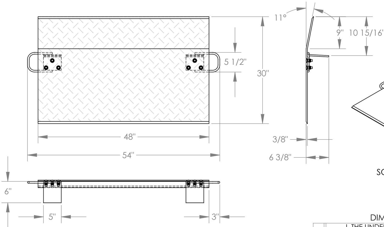
NOTE: BEND OR CROWN IS 11° AND LOCATED 9" FROM EDGE OF DOCKPLATE
