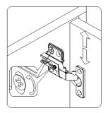
1. Adjust the screws shown in Figure 1 to adjust the door sup and down.
