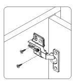
4. After the adjustment is complete, install the remaining two screws to secure the door in place.
