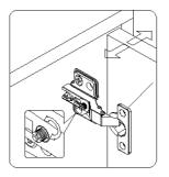
2. Adjust the screws shown in Fig. 2 and pull the door backand forth so that it can be opened smoothly.
