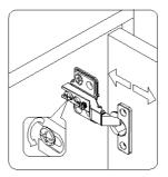
3. Adiust the screws shown in Figure 3 to adjust the door left and right to the right position.
