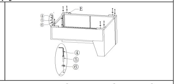
Attach the Foot(E) to the Chair using Bolts(⑤) and Washer Rings(⑥) with Allen Key(④).
