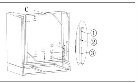
Attach Seat(C) between the Right Armrest(A) and Back(B) using Bolt(②) and Washer(③) with Allen Key(①) from position # I to # V as shown above.
