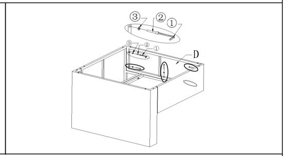
Attach Side Plate(D) between the Back(B) and Seat(C) using Bolt(②) and Washer(③) with Allen Key(①) as shown above.
