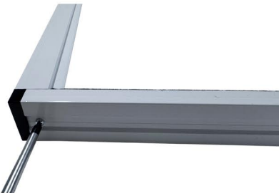
6 The screws were tightened at each of the four corners.
