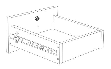
Put it into the reserved holes and tighten the screw
