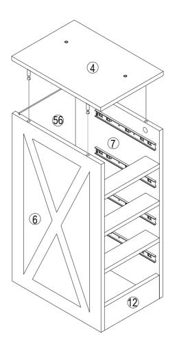
Put it into the reserved holes and tighten the screw
