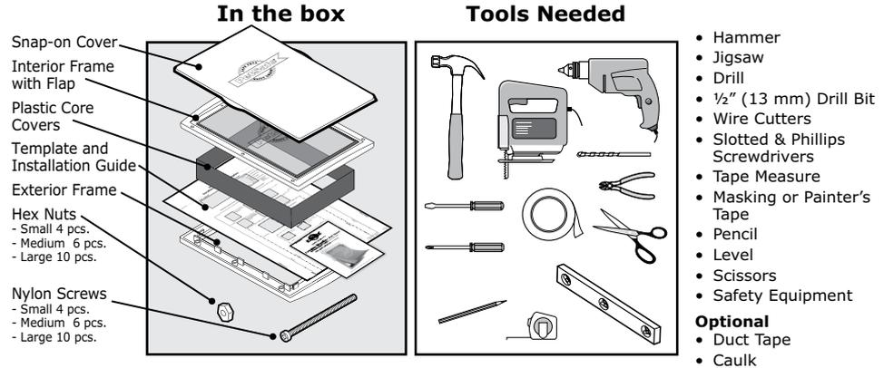
**NOTE:** The Extreme Weather Pet Door™ can be installed in most doors and walls. Installation in thinner or thicker applications may not require the Plastic Core Covers. If installing in a wall, reduce cut-out width by 1" for the Small and Medium. For the Large reduce cut-out width by 1" and cut-out height by 1". Additional tools and materials, such as wood framing, may be required.
