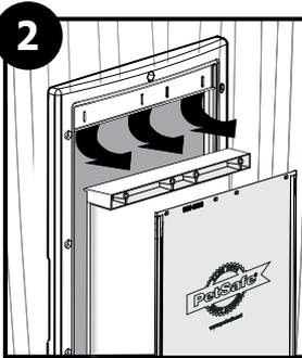
Remove vinyl flap and flap clamp with attached insulated flap.
