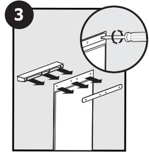
Remove screws, insulated flap and backing plate from back of flap clamp. Insert new insulated flap between flap clamp back and backing plate. Align screw holes. Replace and tighten screws. Follow step 3 under "Vinyl Flap Replacement and Adjustment" on page 9.
