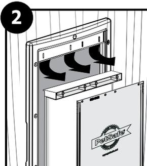
Remove vinyl flap and flap clamp with attached insulated flap.
