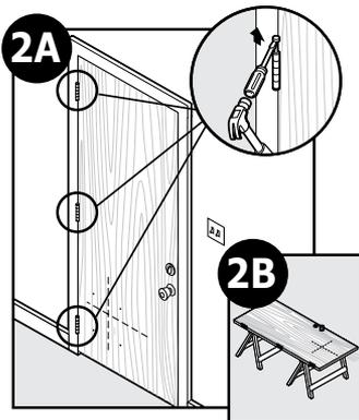
**2A** Remove door by removing door hinge pins.
