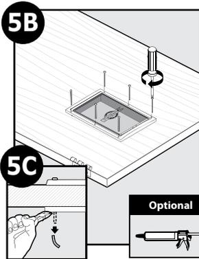
**5B** Use a screwdriver to evenly tighten screws through-out frame while keeping core covers in position. It may be necessary to adjust screws to make sure pet door fit is correct.
