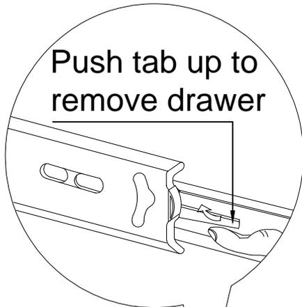
To remove drawer, simultaneously pull
