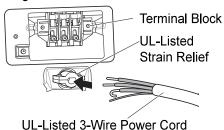
5 Attach the two hot leads (black and red) of the power cord to the outer terminal block screws.
