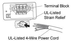
Transfer the dryer's ground wire from behind the green ground screw to the center screw of the terminal block.
