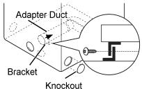
3 Preassemble a 4-inch (10.2 cm) elbow to the next 4-inch (10.2 cm) duct section, and secure all joints with duct tape. Be sure that the male end of the elbow faces AWAY from the dryer. Insert the elbow/duct assembly through the side opening and press it onto the adapter duct. Secure it in place with duct tape. Be sure that the male end of the duct protrudes 1.5 inches (3.8 cm) to connect the remaining ductwork. Attach the cover plate to the back of the dryer with the included screw.
