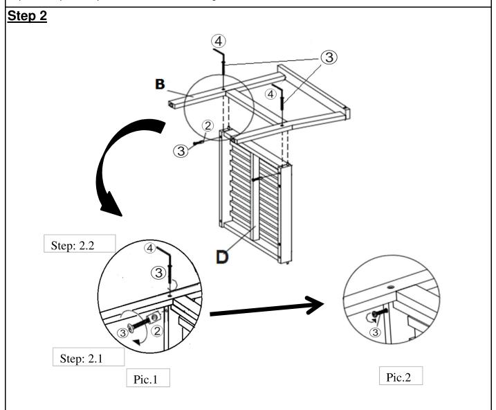
Position Seat Panel (D) and Right Arm Panel (B) as shown in picture above.
