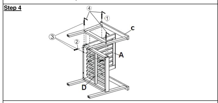
With the help from your partner, turn the Chair to rest on Right Arm Panel (B) so that Left Arm Panel (C) is now facing skywards. Repeat the same process by affixing Screw (1), Cross Nuts (2), Bolts (3) to designated points LOOSELY TIGHTEN THE SCREWS up to 80%.
