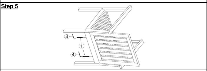
Use Screws (1) and Allen Key (4) to attach Backrest Panel (A) and Seat Panel (D). **LOOSELY TIGHTEN THE SCREWS up to 80%.**
