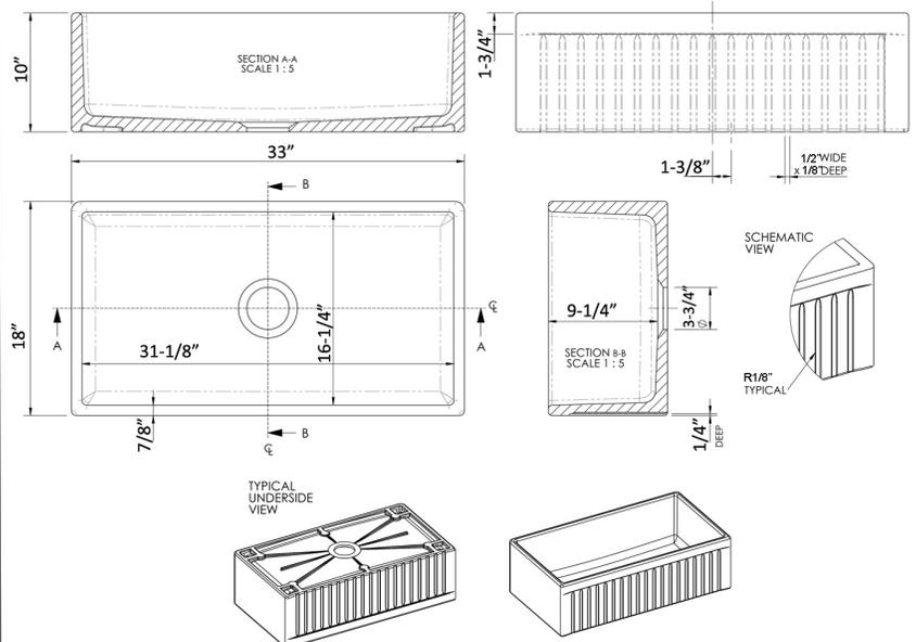
Dimensions of fixture are nominal and may vary within the range of tolerances established by ANSI Standard A112.19.2. Dimensions and specifications subject to change without notice.
