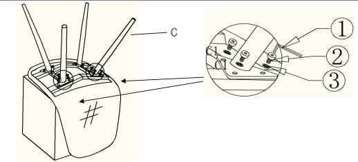
Align the Hind Legs(C) with mounting positions on the base of the Seat(A).
