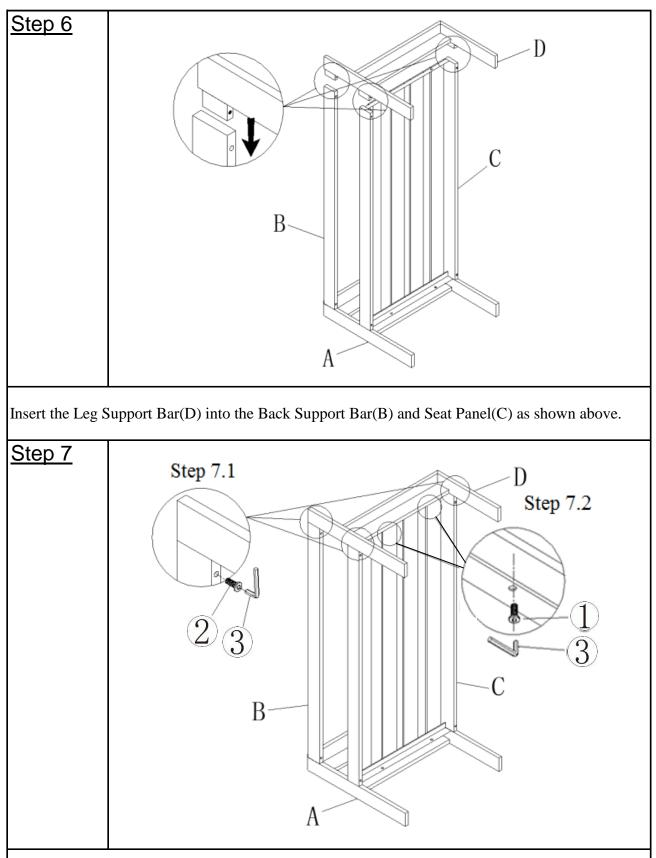
**7.1**) Attach the Leg Support Bar(D) to Back Support Bar(B) and Seat Panel(C) using Bolts(2) with Allen Key(3) as shown above.
