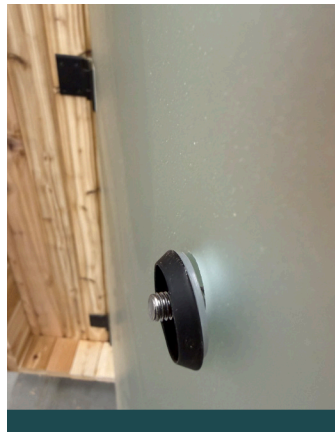
21. Place the plastic washer over the thread on the reverse side of glass and then the metal grommet, followed by the handle with wood spacer.
