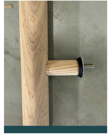
19. Find the handle parts (handle, screw, wood spacer, metal grommet and plastic washer) and assemble as shown, with plastic washer between glass and metal grommet.
