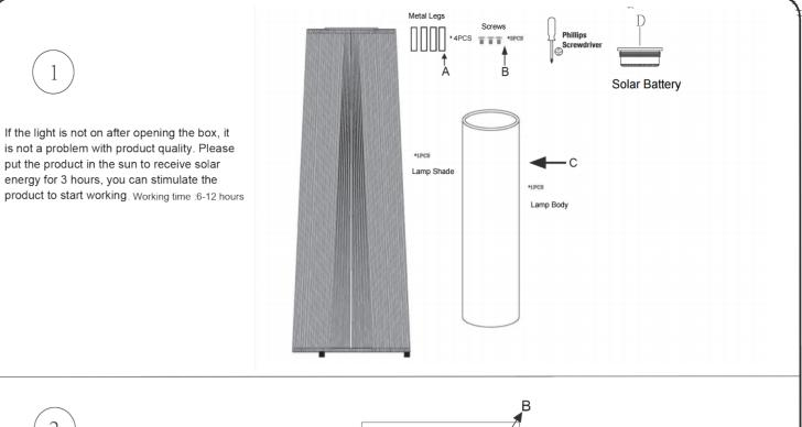
Insert the acrylic lamp body (C) into the lamp shade (E) as shown, use the screw to fix the lamp body.
