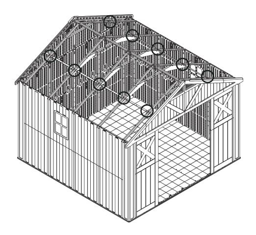
1. Place one end of the 10-D2-7 into the corresponding position and tilt the other end into place.
