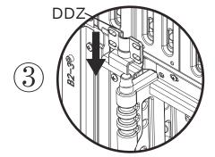
Tilting the **door** and snapping it into the DDZ.
