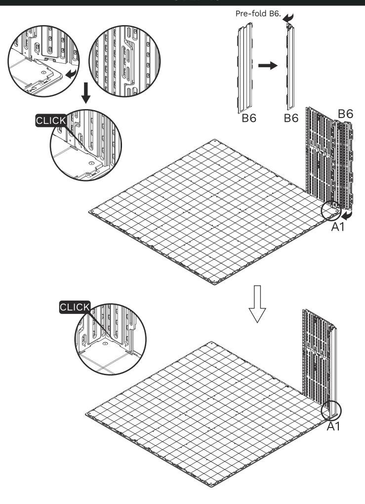
Place the assembled 10-B2 and 10-B1 at the corresponding position on the floor and rotate them into the groove.
