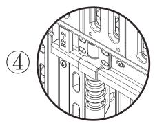
After inserting the DDZ, push the **door** to the fitting position.
