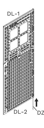
Do not push in hard when there is an obstruction, rotate DZ to adjust.
