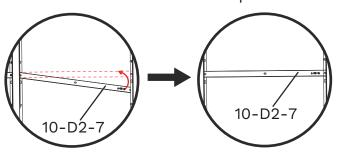
2. Once the holes are aligned, install M6-25 and M6.
