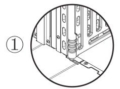
Push it into the groove of the floor.
