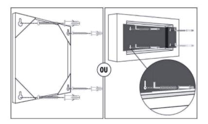
Wall mounting: After having made a location plan at the back of the fireplace, you know the distance of the wall plugs, which must be attached to the wall. Once the wall plugs are attached, just pass the screw heads in the round part of the support, then descend down the fireplace slightly so that the screws take in the widest part of the support. (The supplied wall plugs are only to be used for a concrete wall).
