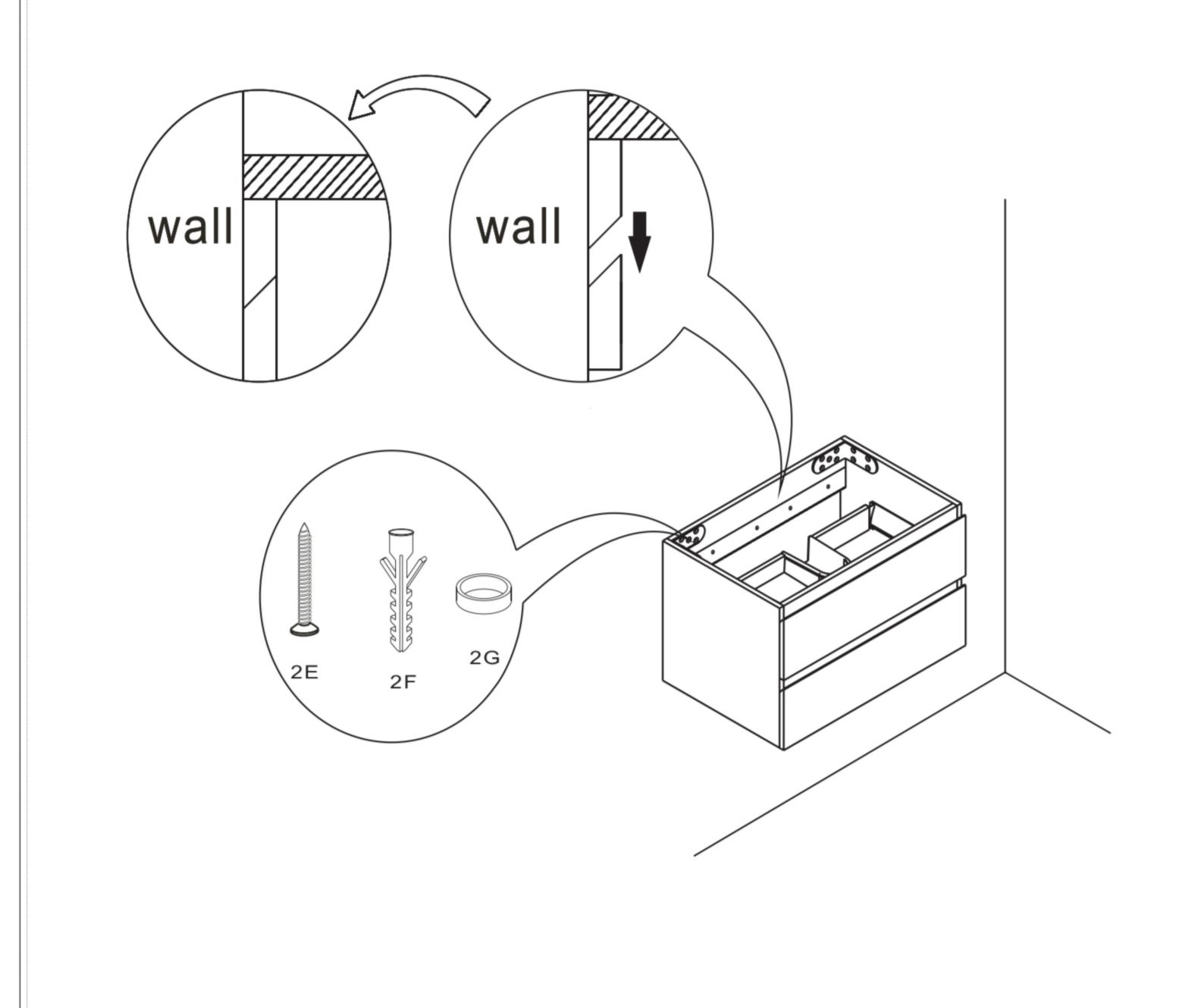
Please fix the cabinet with M6x65 screws which included in the hardware pack, make sure the screw were installed on the wooden stud of the wall.
