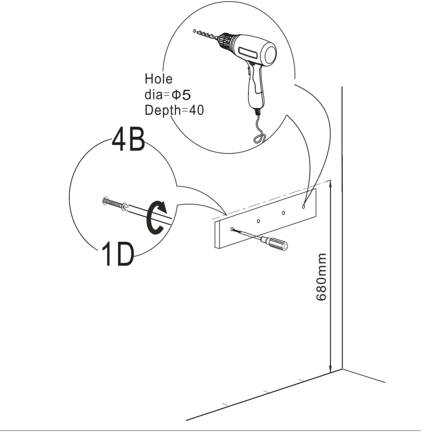
Please make sure to install screws on the wooden stud of the wall to help stabilize.
