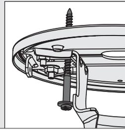
Use the wood screw to poke holes through the rubber gasket in order to install the ceiling bracket assembly to your support structure or ceiling fan-rated outlet box.
