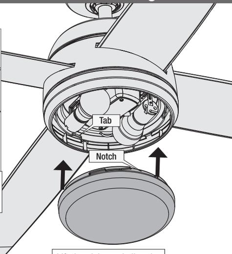
Lift the globe and align the notches in the globe with the tabs in the light kit.
