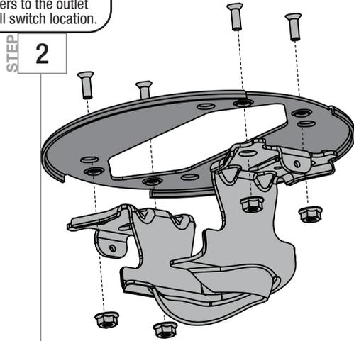
Align the tapered mounting holes in the ceiling plate with the holes in the ceiling bracket. Install the four ceiling plate screws found in the hardware bag and secure with the flange nuts using an 11/32" wrench. Hold the ceiling bracket assembly up to the outlet box and mark the screw locations. To mount to support structure, also mark the ceiling for drilling pilot holes.
