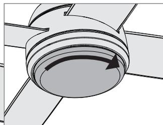
Attach the globe by lifting and turning clockwise one third of a full turn of the glass until it stops.
