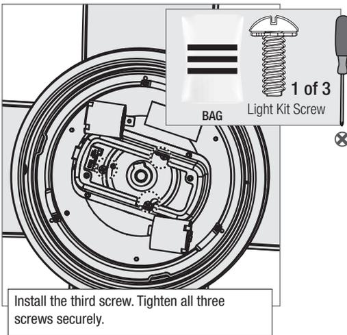
Install the third screw. Tighten all three screws securely.
