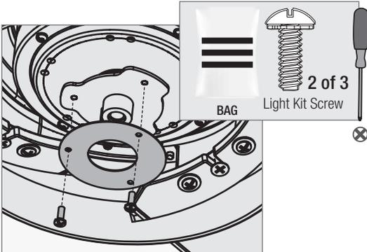
Partially install two light kit screws, found in the hardware bag, through the gasket halfway into the motor housing as shown. It does not matter which two screw holes you choose.
