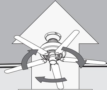
Updraft (clockwise rotation) creates a more indirect airflow. Updraft airflow is great for moving warm air downward.
