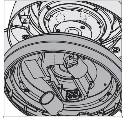
Align the keyhole slots in the top of the upper switch housing with the partially installed light kit screws. Wrap the keyhole slots around the screws and twist counterclockwise
